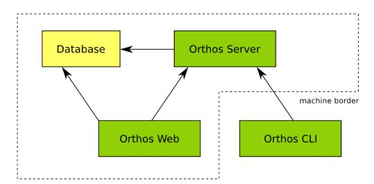
Image Overall Architecture shows the overall architecture. All data is kept in the database. The Orthos Server is the central component of Orthos. It has the following tasks:
